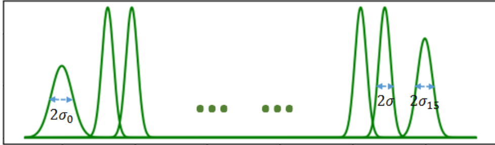
Figure 3-8: Flash channel model with 16-ary signal constellation. Note S_0 and S_{15} have higher variance. The separation between these two symbols and the other symbols is relatively high to balance out the raw error rate and maximize the channel capacity. The dots represent the rest of the 16 symbols with variance \sigma . Note the labels on the figure are twice the variance.
