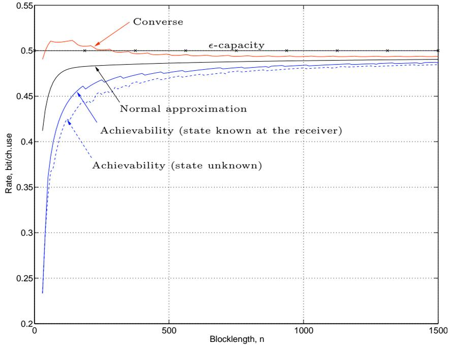
Fig. 5. Rate-blocklength tradeoff at block error rate  $\epsilon = 0.03$  for the non-ergodic BSC whose transition probability is  $\delta_1 = 0.11$  with probability  $p_1 = 0.1$  and  $\delta_2 = 0.05$  with probability  $p_2 = 0.9$ .
