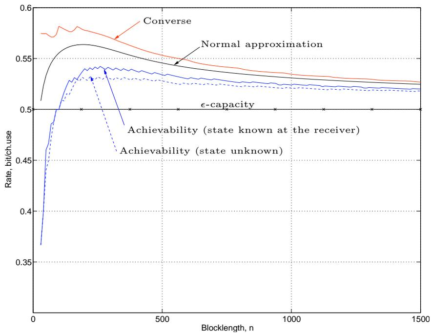
Fig. 6. Rate-blocklength tradeoff at block error rate  $\epsilon = 0.08$  for the non-ergodic BSC whose transition probability is  $\delta_1 = 0.11$  with probability  $p_1 = 0.1$  and  $\delta_2 = 0.05$  with probability  $p_2 = 0.9$ .
